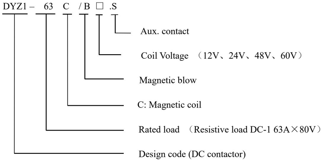
Example: DYZ1-63 - c/B60. S. indicates Magnetic latching DC contactor, rated current at DC-1 load is 63A, coil voltage is DC60V. Products with magnetic blowing, with auxiliary contact.
